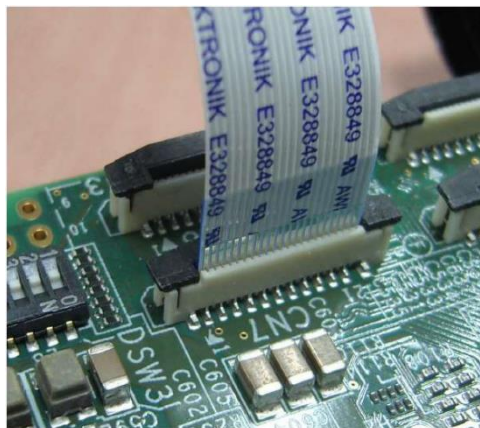
Figure 3.1-2 Connect FFC to RZ/V2H Secure Evaluation Board.
