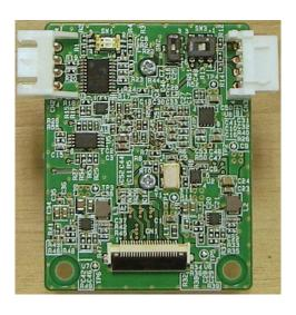
Figure 2.2-5 IMX415 Board-M12 (V2HEVK connector side)
