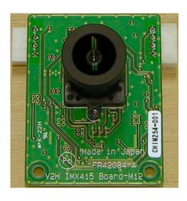
Figure 2.2-4 IMX415 Board-M12 (IMX415 sensor side)
