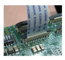
Figure 3.1-2 Connect FFC to RZ/V2H Secure Evaluation Board.
