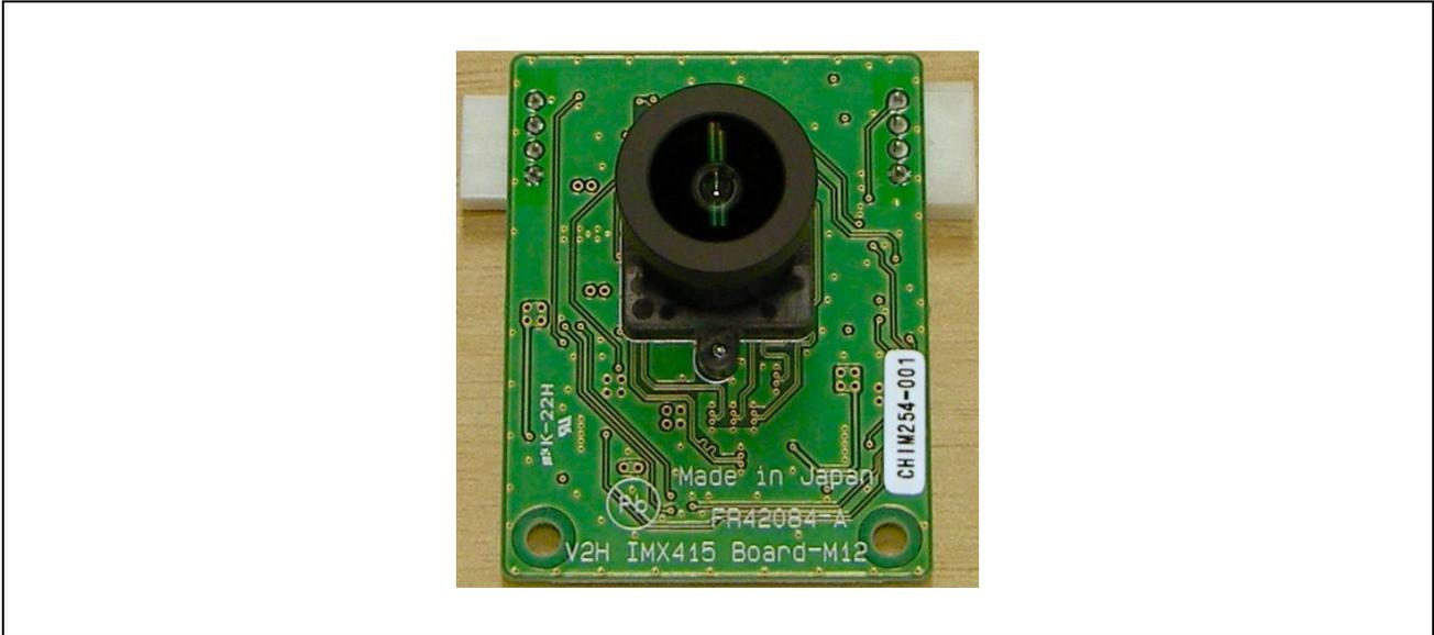
Figure 2.2-4 IMX415 Board-M12 (IMX415 sensor side)
